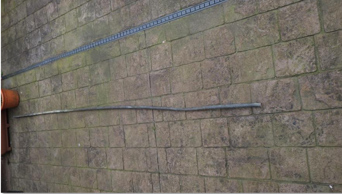
Figure 6.11 Probable brass condenser tube 240 cm x 2 cm (Source: C Holden)
