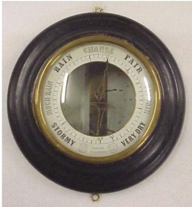
Fig 20 The 20cm aneroid barometer, in a black wood case, salvaged from the SV Maria Borges Photo courtesy of the Mariners Museum and park, Newport News, Virginia
